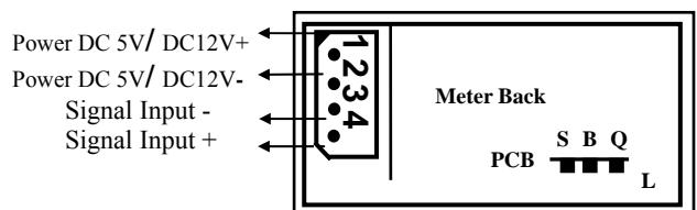
PIN 1: Power DC 5V/ DC12V+ (Positive pole)
